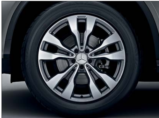
5-twin-spoke light-alloy wheels, painted vanadium silver with a high-sheen finish, with 275/50 R20
